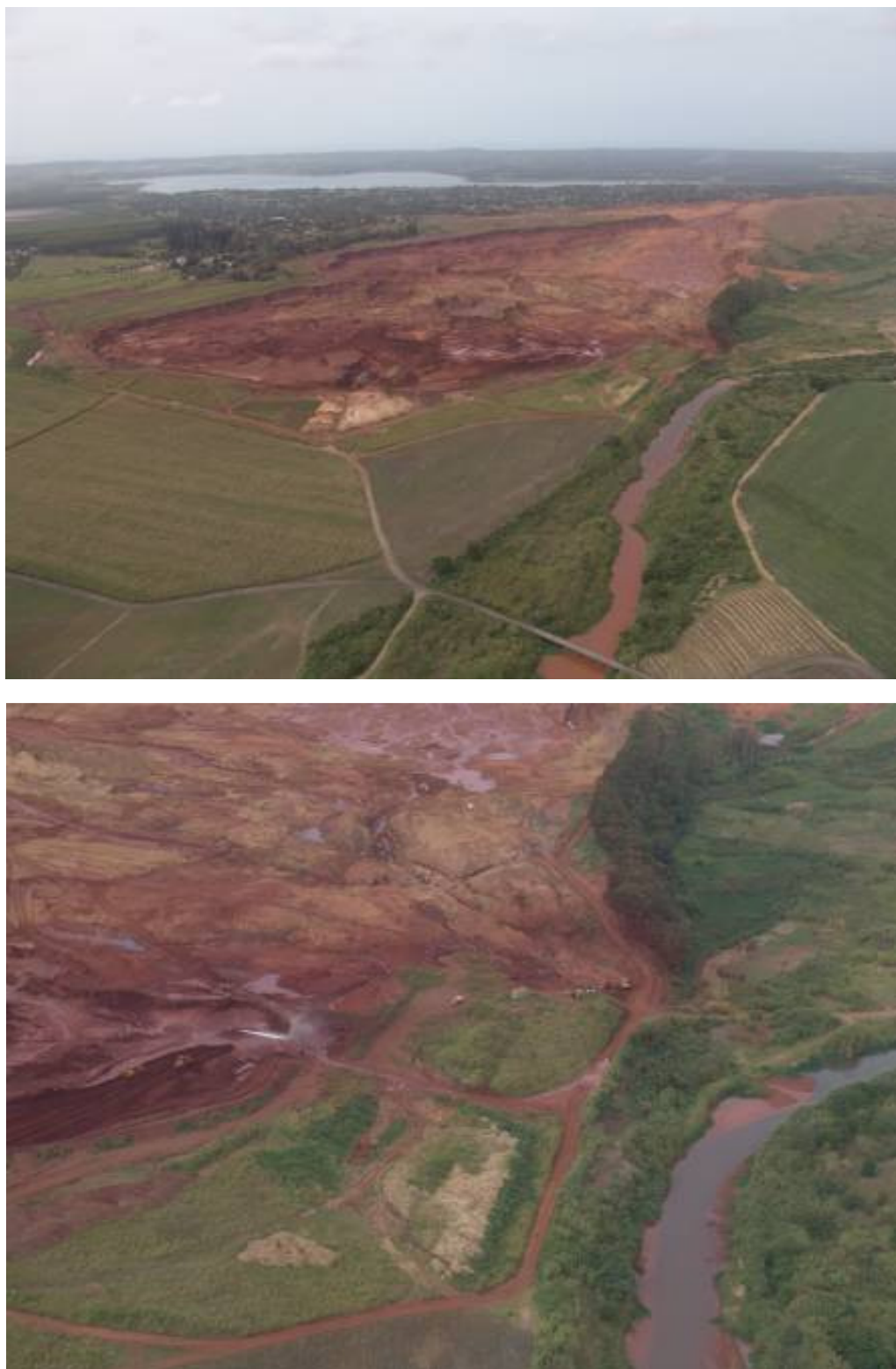
Figure 7: Mining operations at Hillendale. Note the formation of an "alluvial fan" in the uMhlathuze river (bottom photograph), which is the result of sand being washed into the river.
